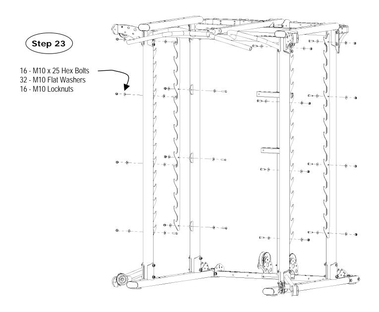
Step 23: Attach the four Weight Rack Plates onto the outer sides of the mounting tabs on the Main Uprights with the "Hooks" pointing up using:
