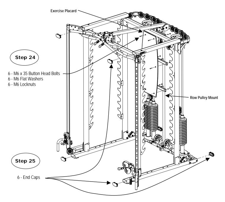
Step 24: Attach the Exercise Placard to the Row Pulley Mount using:
