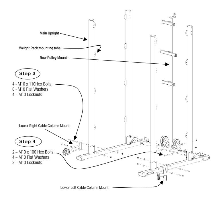
Step 3: Attach the two front Main Uprights, Lower Right Cable Column Mount, and Lower Left Cable Column Mount to the Left and Right Base Beams using:
