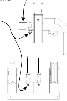
Readjust the cables with the Cable Bolts to remove any new slack. If after readjusting the cables there is still excess slack, you can adjust more slack out by moving the clevis on the end of the Lower Cables to the lower hole in the Cable Anchor.
