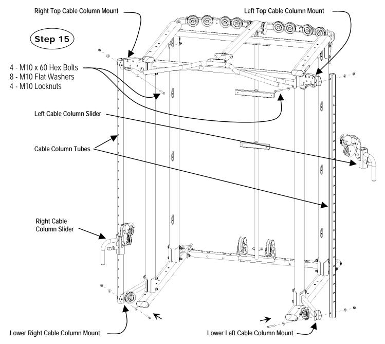
Step 15: Identify one of the Cable Column Tube's upper end, (the end with the slotted holes). Assemble the Right Cable Column Slider onto the Cable Column Tube. Make sure the Pop-pin aligns with the holes in the tube. Attach the Right Cable Column Tube Assembly to the Right Upper and Lower Cable Column Mounts using:
