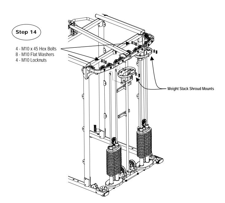
Step 14: Install the two Weight Stack Shroud Mounts. One at a time, position the Weight Stack Shroud Mounts at the top of the Guide Rod pairs. Slide these down the Guide Rods and secure in position using:
