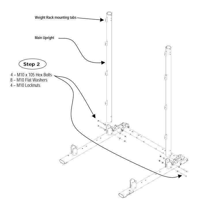
Step 2: Attach two Main Uprights to the rear of the Left and Right Right Base Beams (orient all Uprights with the four Weight Rack mounting tabs toward the middle of the machine and near the top) using:
