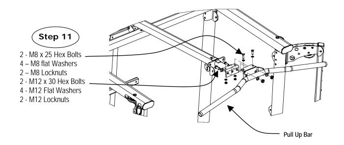
Step 11: Attach the Pull-Up Bar to the Lat Attachment using:
