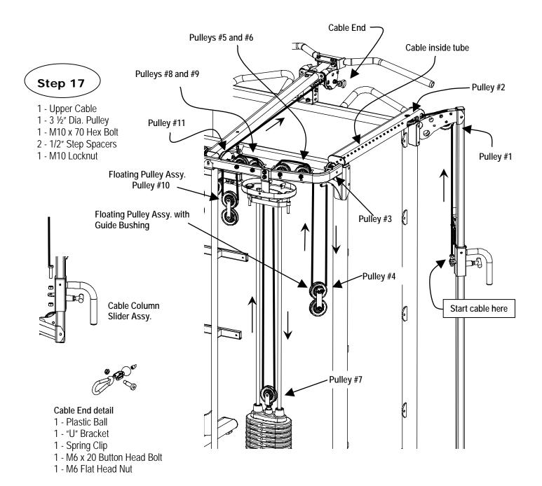
Step 17: Install the Upper Cable on the right side of the machine. Repeat the installation sequence in Step 16, but this time on the right side of the machine using:
