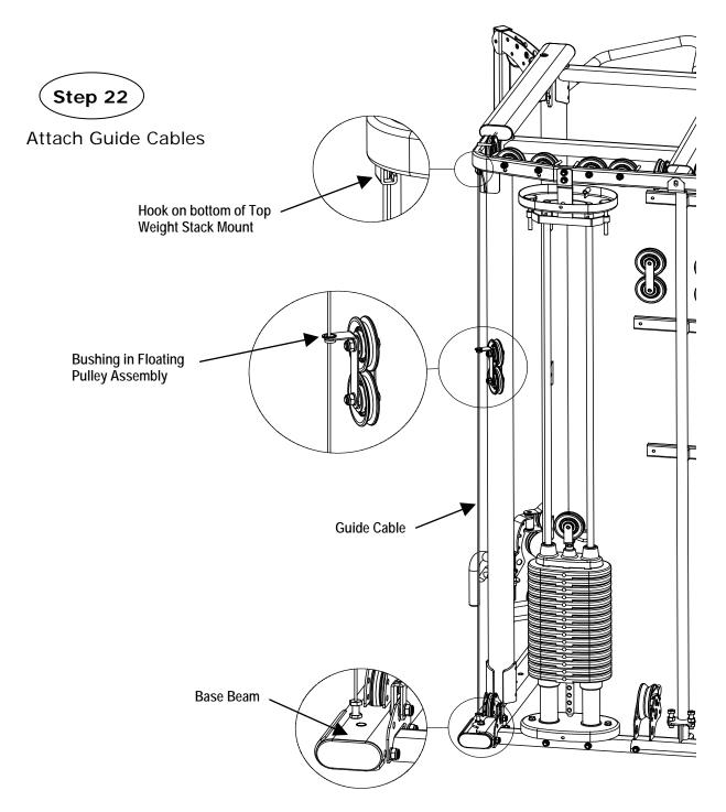
Step 22: Feed the small end of the Guide Cable up through the bushing in the Floating Pulley Assembly and attach the end to the hook on the bottom of the Top Weight Stack Mount. Insert the bolt end into the threaded hole in the Base Beam. Tighten the bolt so the Guide Cable is taught, but do not over tighten. Tighten the jam nut.
