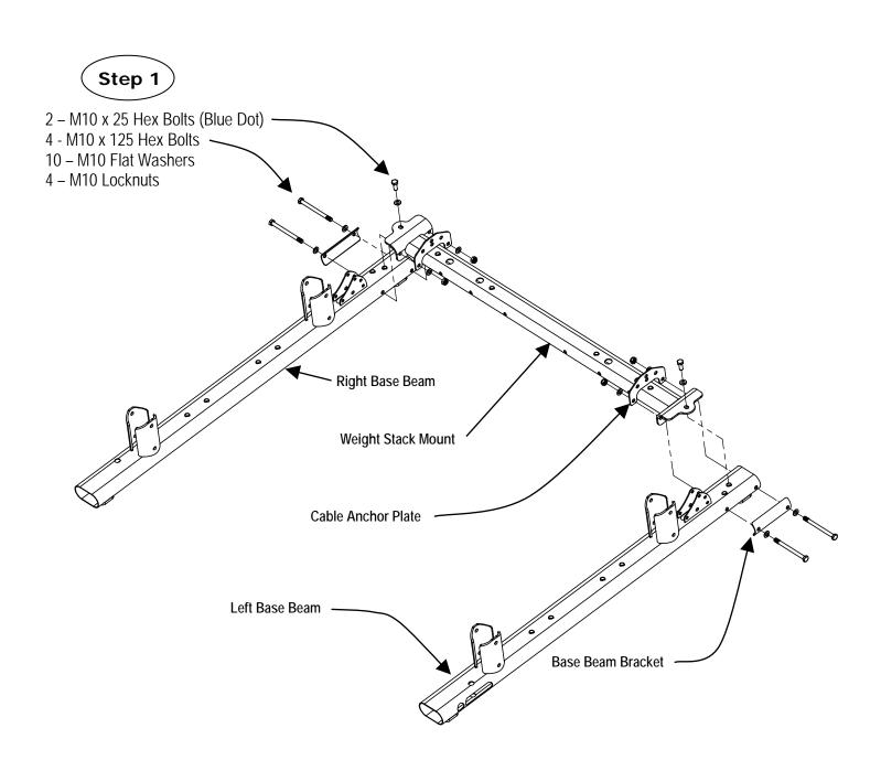
Step 1: Attach the Right Base Beam, Left Base Beam, Weight Stack Mount, two Cable Anchor Plates, And two Base Beam Brackets using:
