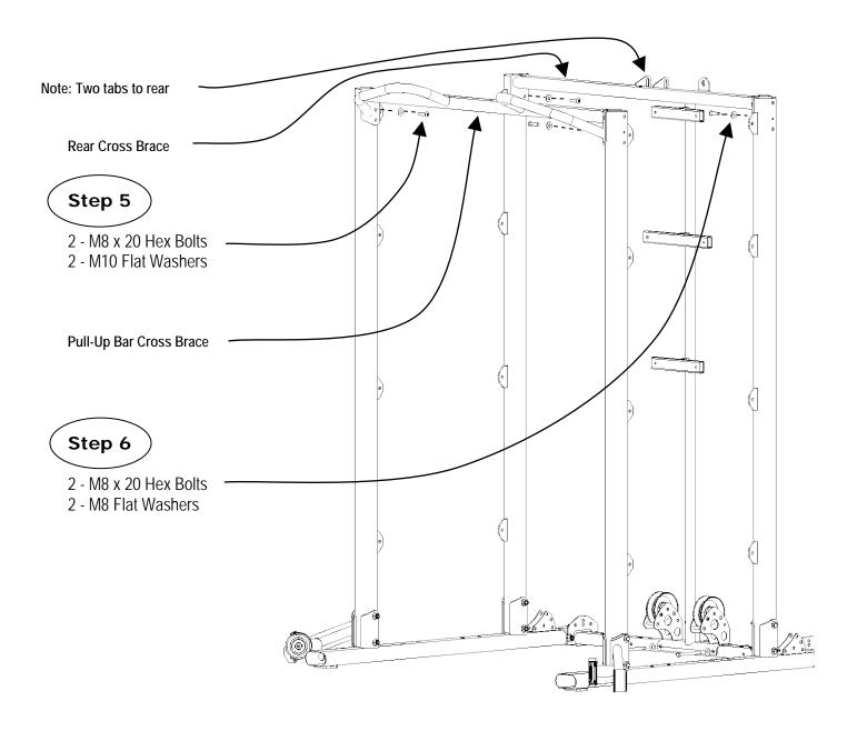
Step 5: Attach the Pull-Up Cross Brace to top of front Main Uprights using:
