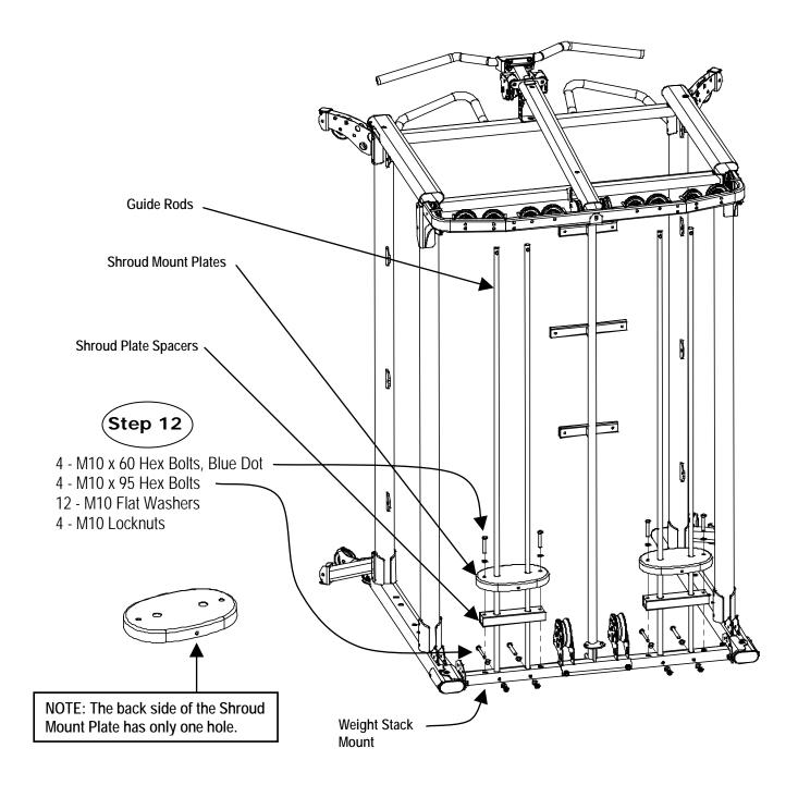
Step 12: Attach four Guide Rods to the Weight Stack Mount using:
