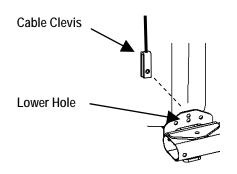
If after adjusting cable length(s) as noted above and the cable appears to be too short, remove the Top Weight Pulley, screw out the "U" bracket one to two full turns, then retighten the Jam Nut, and re-attach the pulley. Make sure the Locknut on the Pulley bolt is facing toward the back of the cage.
