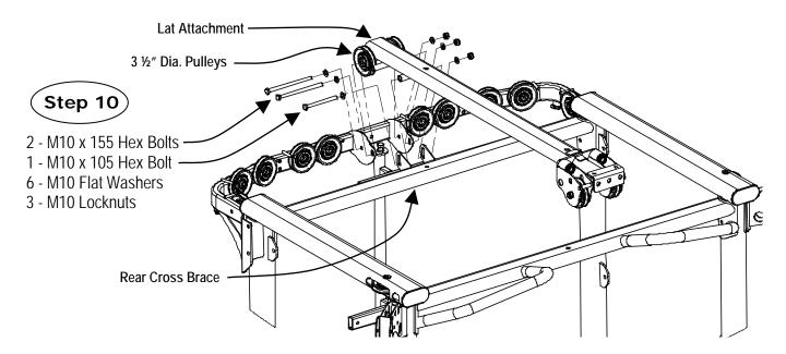
Step 10: Assure the M12 Hex Bolt from STEP 9 is installed in the top of the Row Pulley Mount and adjusted to the minimum height. Attach the Lat Attachment and two 3 ½" diameter pulleys to the top of the Weight Stack Mount and Rear Cross Brace using:
