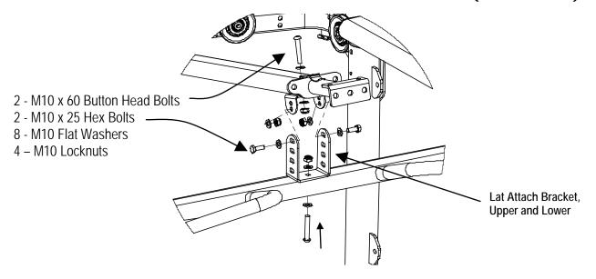
Now install two Brackets supporting the Lat Attachment to Pull Up Cross Brace with the Button Head Bolts, pointing up through the Pull Up Cross Brace. Use M10 x 60 Button Head Bolts with the locknut on top of the Lat Attachment. Use the M10 x 25 Hex Bolts to secure the height adjustment of the brackets together using:
