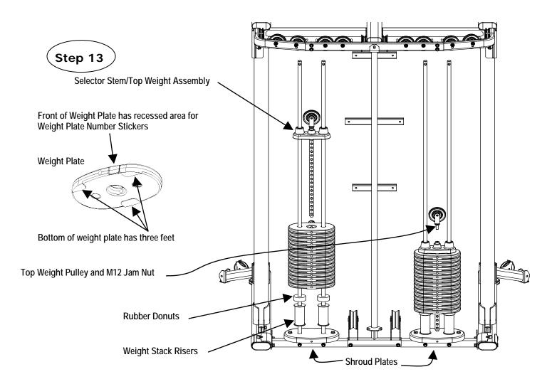
NOTE: Before beginning Step 13: If optional 200 lb. heavy stack is being assembled, eliminate the Weight Stack Risers. This space will be taken up by 5 extra Weight Plates.
