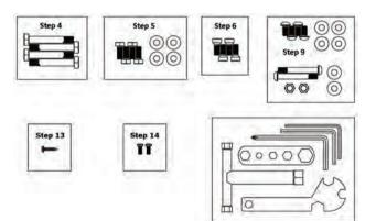
The parts required for each step of the assembly process are sorted by step in individual marked clear plastic bags. Each step has required parts and each of those parts is included with the bag printed with the assembly step.
