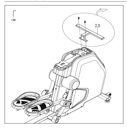
1. Use L Allen Wrench (No.138) to remove two 3/8"x3/4" Socket Head Cap Bolts that hold the protective Side Back (No.23) onto the mounting plate on the Main Frame. Discard the bolts and set the Side Back (No.23) aside.
